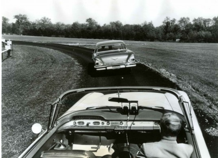
Figure 22: GM and RCA developed and tested smart highways in the 1950s. Magnets in the car tracked a steel cable in the road and control towers managed the traffic regarding speed and steering using radio control.
