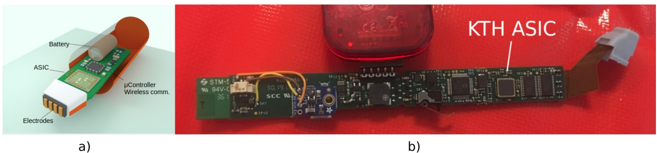
Figure 1, a) Skin cancer detection device, b) product prototype (reproduced with permission of SciBase AB)
