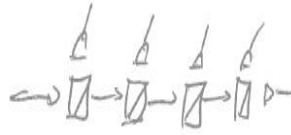
Figure 9.4: Chaining beam splitters and detectors can help to measure photon number to distinguish a one photon state from a two photon state for example.
