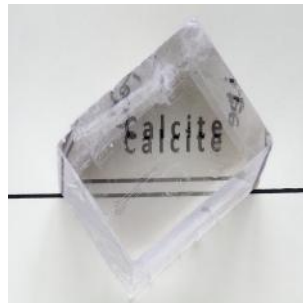
Figure 6.4: A birefringent calcite crystal: different polarizations have different refractive indexes.
