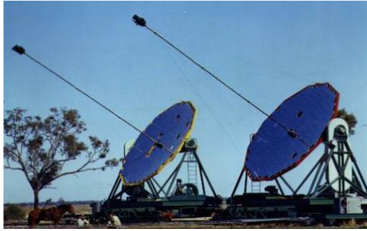
Figure 13.1: Two telescopes focus incoming light from a distant star. Correlation measurements between the two detectors yields the angular size of the star. The resolution is equivalent to a telescope with an aperture equal to the distance between the two telescopes.
