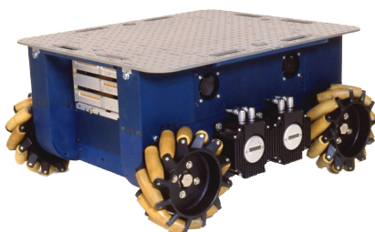
Figure 2.7: An example of an omni-directional platform using mecanum wheels [18]
