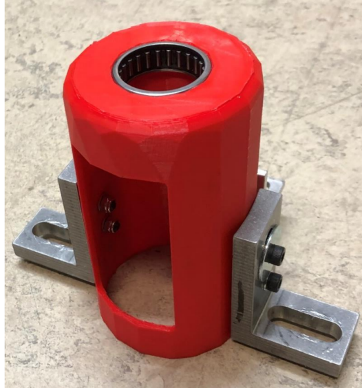
Figure 24: Inline transducer sleeve designed by Adam Klotblix and Sofia Olsson.[49]
