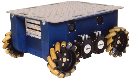
Figure 3.8. An example of an omni-directional platform using mecanum wheels [20]
