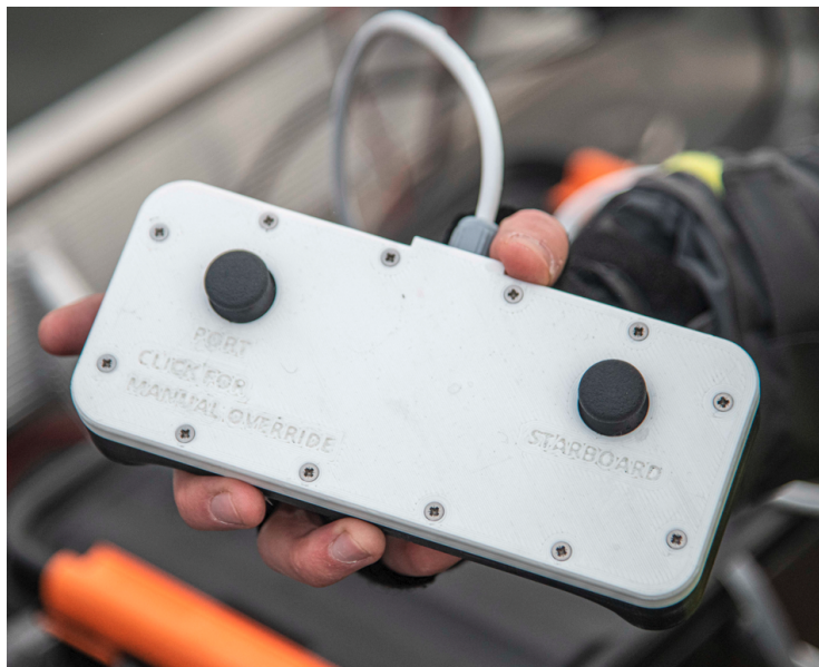
Figure 5.14. Joystick controller used to manually override autonomous system.
