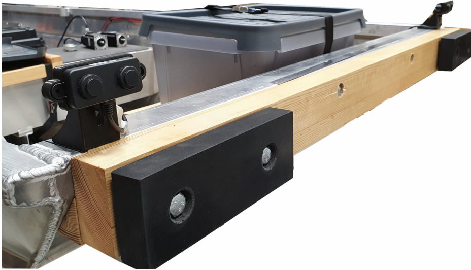
Figure 5.28. Image of the completed bumper assembly with ultrasonics mounted above.
