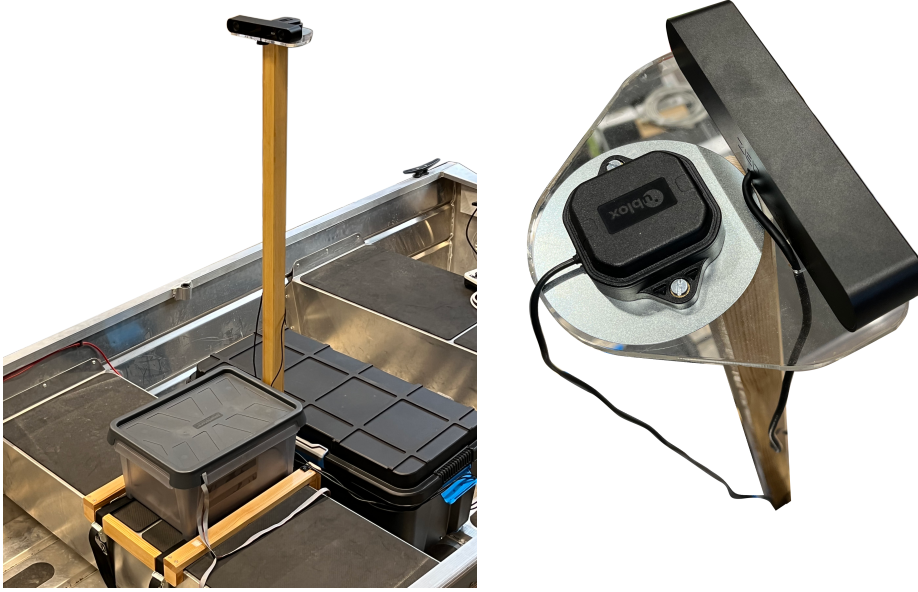
Figure 5.23. Left: Complete mast assembly. Right: Mounting plate on mast with GNSS-antenna and ZED 2 stereo camera.
