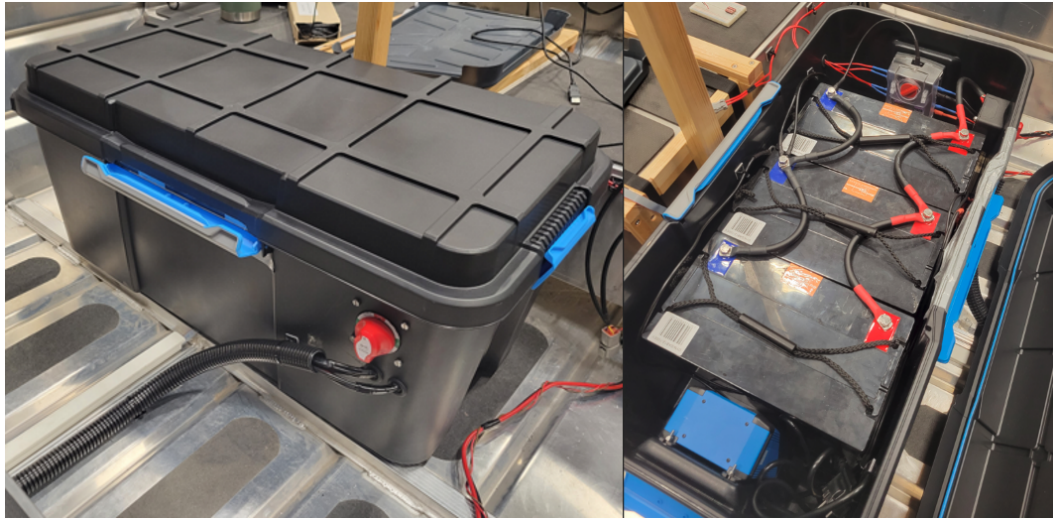
Figure 5.12. Accumulator enclosure including AGM batteries, power switch, fuse box, and charger.
