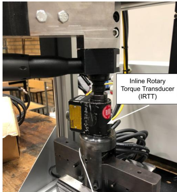
Figure 28: Height adjustment enables the rig to fit an IRTT sensor
