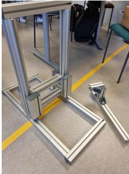
Figure 25: The frame of the test rig, built by aluminium profiles.
