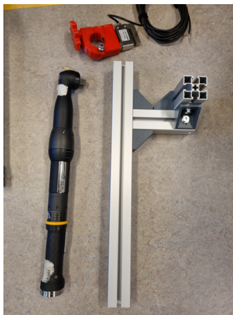
(a) A nutrunner and components used to build the tool arm.
