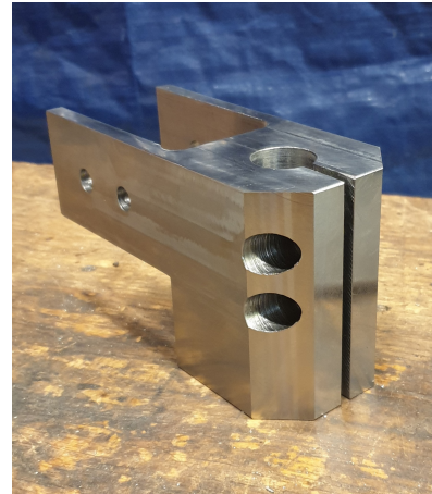
(b) The machined custom adapter.
