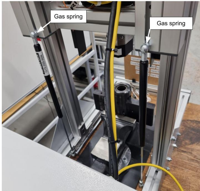
Figure 30: Two gas cylinders decreasing the weight on the tool and beam test joint.
