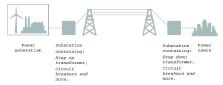
Figure 26: Very simplified picture of the power grid in which breakers and transformers are a part.
