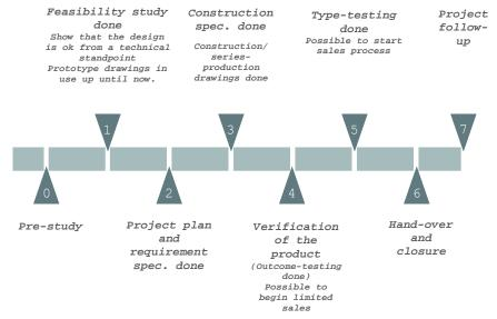
Figure 28: The stage-gate model used for the Breaker development project
