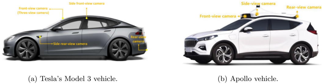
Figure 6: Cameras configurations in autonomous vehicles [48].
