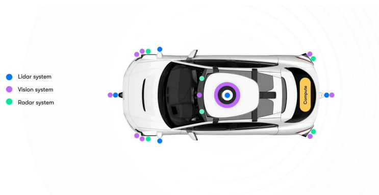
Figure 5: Sensors configuration in a Waymo vehicle [57], edited with [2].
