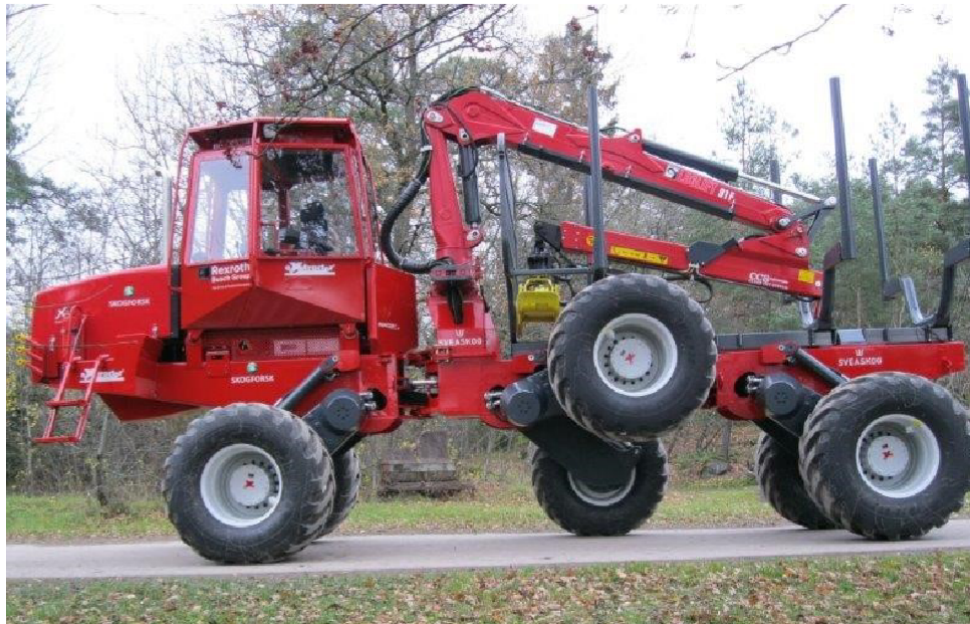
Figure 17: Active pendulum suspension on the XT28 showing ability to control each wheel individually.
