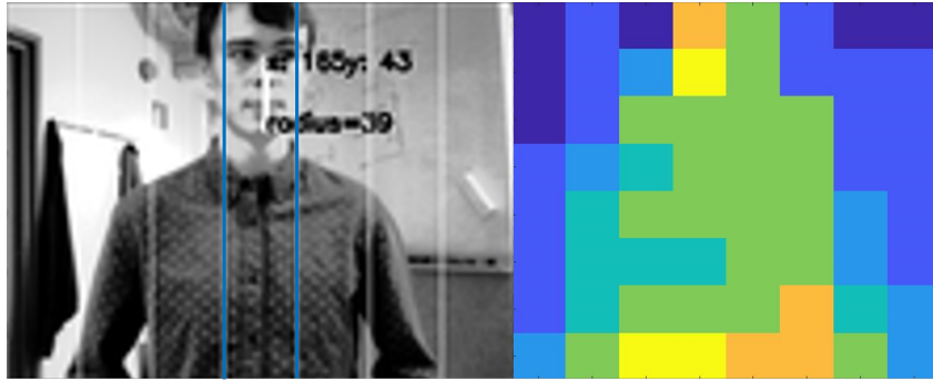
Figure 5.15. A side-by-side comparison of how the robot sees a person in front of it. Photos by authors.
