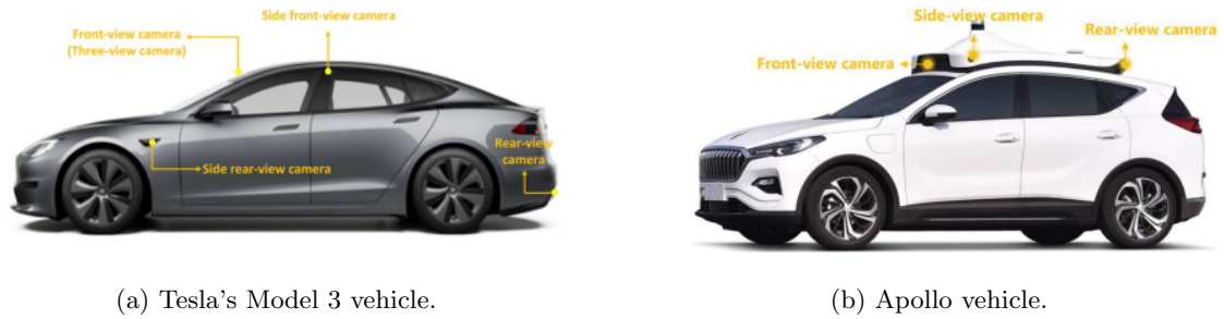
Figure 6: Cameras configurations in autonomous vehicles [58]
