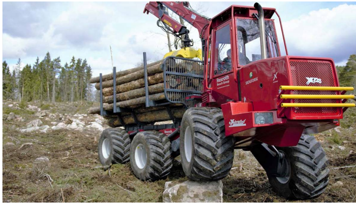
Figure 8: XT28 climbing over a rock
