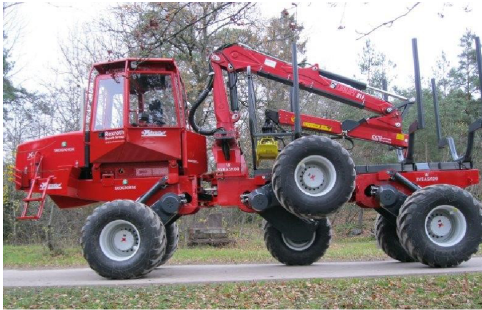
Figure 14: Active pendulum suspension on the XT28 showing ability to control each wheel individually.
