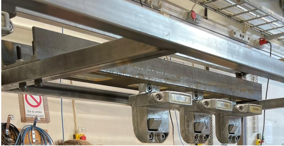
Figure 6.3: The manufactured prototype magazine, mounted to the frame and with twistlocks attached
