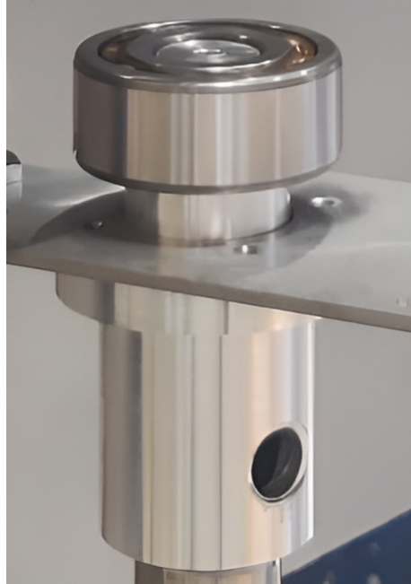
Figure 6.4: The \phi -axis actuator mount adaptor mounted on the Y-axis actuator, \phi -axis actuator mount and bearing
