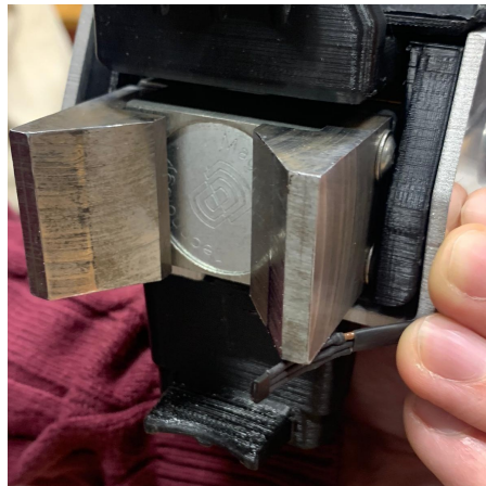
Figure 6.5.: One working position of the hall effect sensor, right below the rightmost pole shoe in the image.
