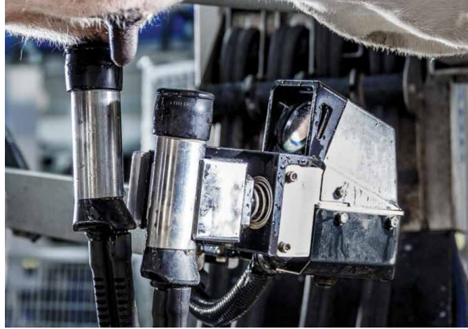
Figure 2.2.: DeLaval AMR magnetic Gripper, ©2023 Delaval. Reprinted with permission from [8].
