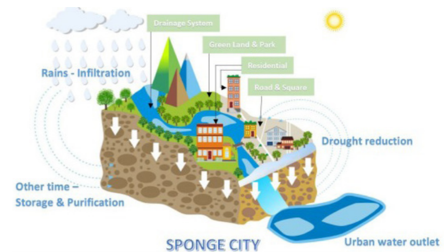
Schematic diagram of the "Sponge City" concept (Chan et al. 2018)
