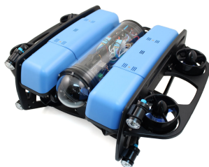
Figure 2.1: BlueROV2 with 8-thruster setup
