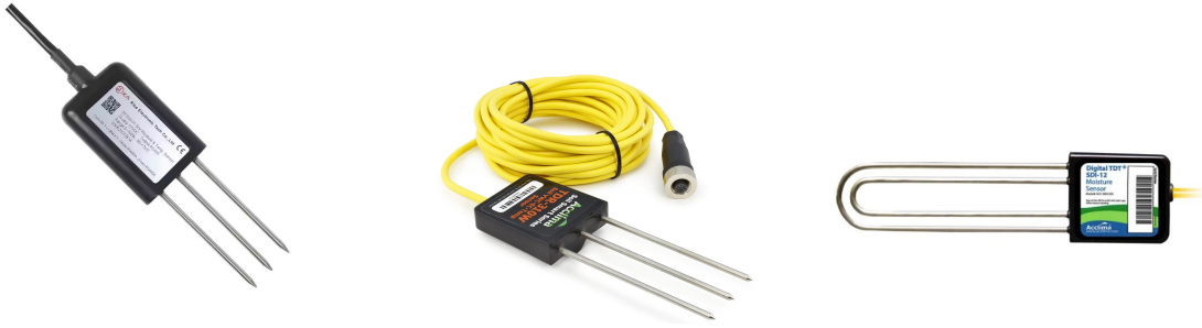
Figure 1: Visual representation of a typical moisture sensor. FDR, TDR and TDT respectively.
