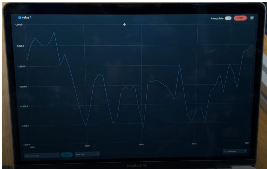
Figure D.1: Graph showing load cell signal during vibration testing.
