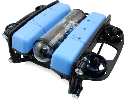
Figure 3.1: Standard BlueROV2 Heavy Configuration
