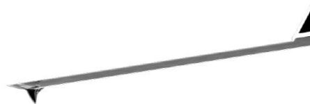
Right: cantilever, 228 \mu\text{m} long micro-fabricated silicon cantilever with integrated tip.
