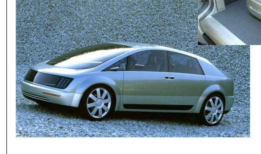
Skateboard concept Fuel cell 94kW Integrated distributed control Weight: 2 tons, Distance: 480kn
