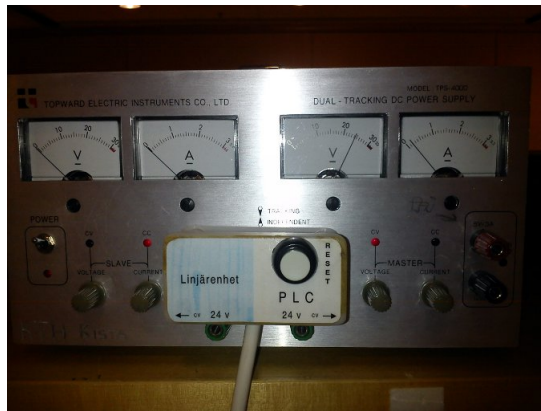
Figure 6: PLC power connected to DC power supply
