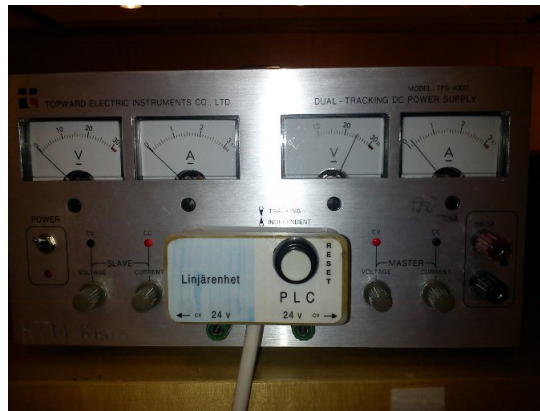
Figure 6: PLC power connected to DC power supply
