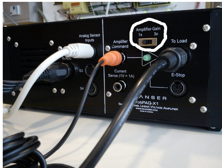
Figure 5: Amplifier Gain should be set to 1x.
