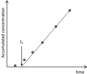
In a diffusion experiment a 1.0 cm long diffusion cell packed with 1.41 grams bentonite clay (which gave a dry density of 1.8 g/cm<sup>3</sup>) is used.  $\Gamma$  is the ion to be studied and the inlet solution contains 10 mM NaI spiked with <sup>131</sup>I (which is a  $\beta$ -emitter,  $t_{1/2} = 8.02$  d). Samples are taken at different times from the outlet solution. The samples are measured for activity in a liquid scintillator ( $\eta = 83\%$ ).
