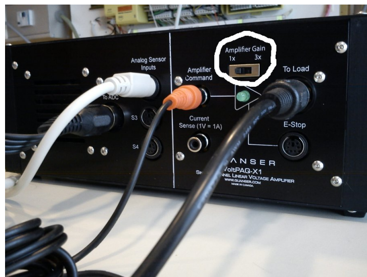
Figure 5: Amplifier Gain should be set to 1x.
