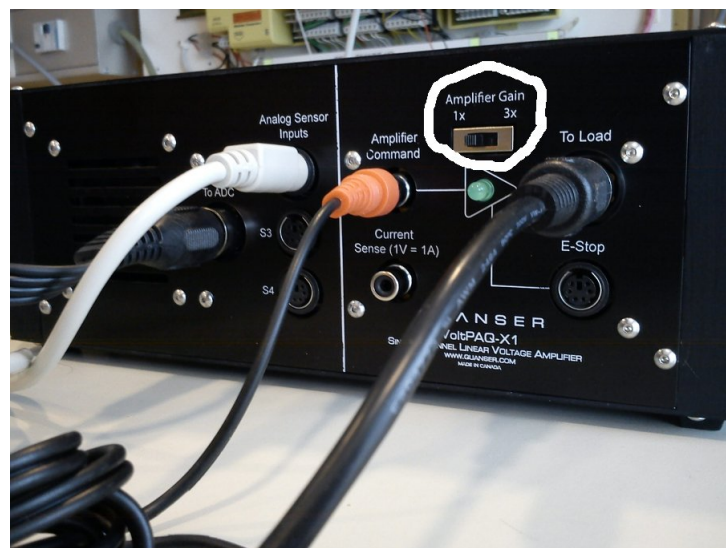
Figure 5: Amplifier Gain should be set to 1x.
