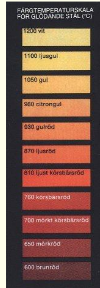
Chart to estimate steel temperature in steelworks.
