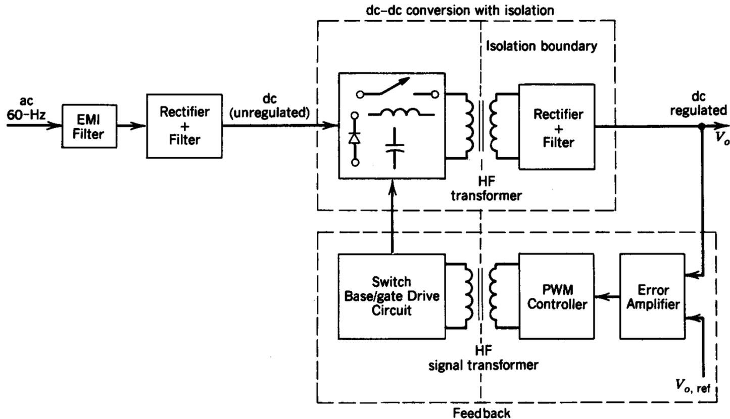
**Figure 10-2** Schematic of a switch-mode dc power supply.
