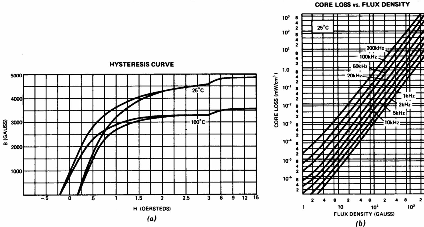
Figure 10-17 3C8 ferrite characteristic curves: (a) B-H loop; (b) core loss curves. (Courtesy of Ferroxcube Division of Amperex Electronic Corporation.)
