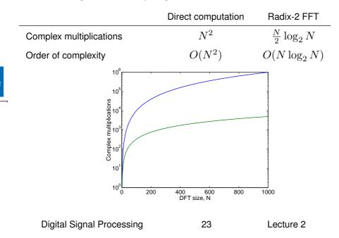
FFT is a *fast algorithm* for computing the DFT.
