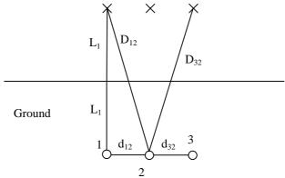
The temperature rise is maximal of the middle conductor, because it has two neighbour conductors that contributes the temperature rise. We then can concentrate on to treat the middle conductor.
