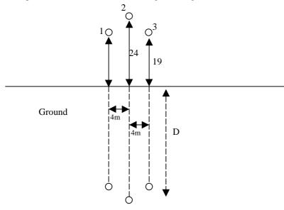
The distance to the mirror image currents, which corresponds to the real phase currents can be calculated according to Carson's formula
