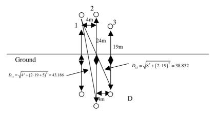
The distances  $d_{12}$ ,  $d_{23}$  and  $d_{13}$  between the conductors are calculated according to
