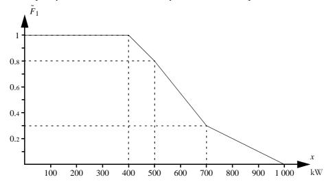
**a) (2 p)** The figure above shows the equivalent load duration curve including outages in the hydro power plant. How large is the expected energy not served per hour if only the hydro power plant is considered?
