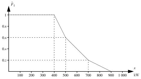
**a) (3 p)** The figure above shows the duration curve of the equivalent load including outages in the hydro power plant. How large is the expected electricity generation per hour in the hydro power plant?
