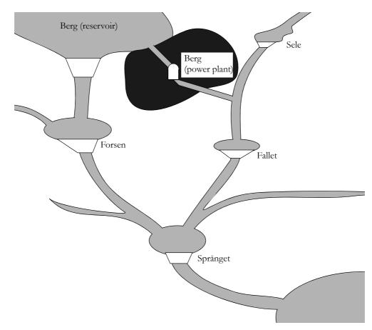
f) (2 p) Consider the hydro power plants in the figure above. Notice that Berg is an underground power plant and water that is discharged through the turbine is flowing to Fallet, whereas spillage goes to Forsen. The water delay time between the power plants can be neglected.
