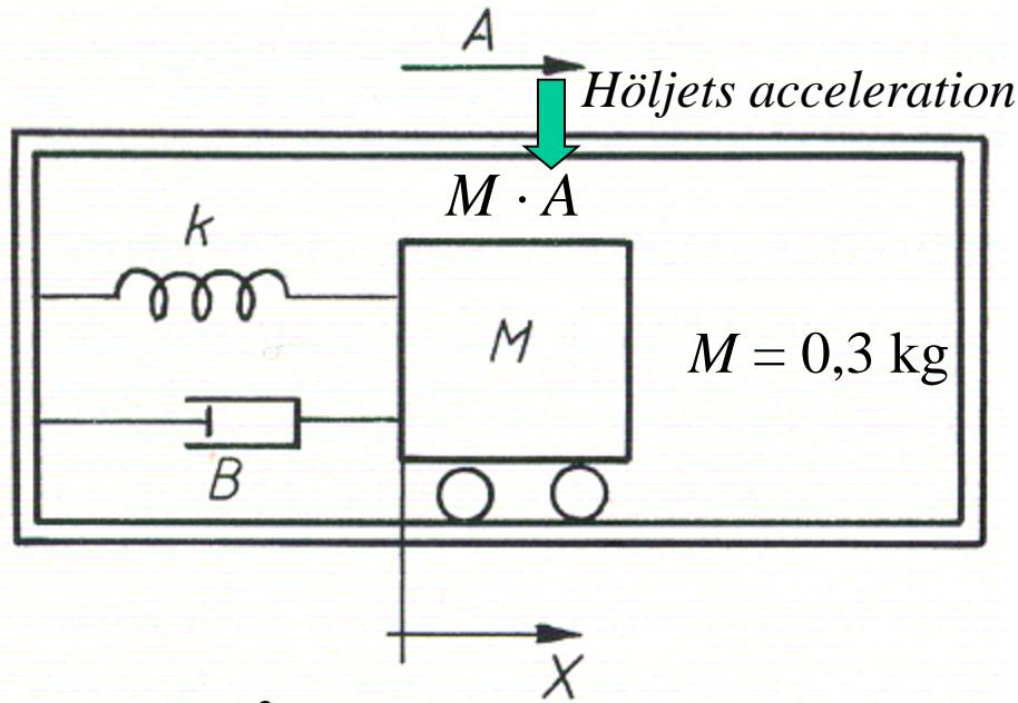
$$M \cdot A + k \cdot x + B \frac{dx}{dt} = -M \frac{d^2 x}{dt^2} \quad \{L:\} \quad MA + kX + BX_s = -MXs^2$$
