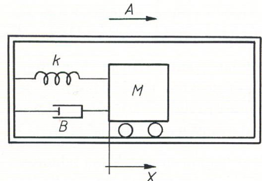
$$G(s) = \frac{K\omega_0^2 \xleftarrow{\text{gain}}}{s^2 + 2\zeta\omega_0 s + \omega_0^2} \quad \zeta = 0,69 \quad M = 0,3 \text{ kg}$$
