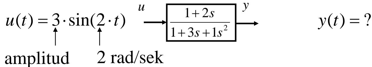
$$\frac{1+2s}{1+3s+s^2} \quad j\omega = s \quad \frac{1+2j\omega}{1+3j\omega+(j\omega)^2} = \frac{1+2j\omega}{1-\omega^2+3j\omega}$$
