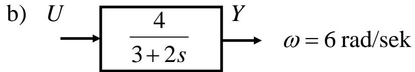
$$A(\omega) = \frac{4}{\sqrt{9 + 4\omega^2}} \quad \varphi(\omega) = 0 - \arctan \frac{2\omega}{3}$$
