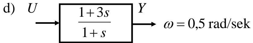
$$A(\omega) = \frac{\sqrt{1+9\omega^2}}{\sqrt{1+\omega^2}} \quad \varphi(\omega) = \arctan 3\omega - \arctan \omega$$
