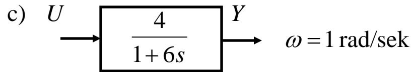
$$A(\omega) = \frac{4}{\sqrt{9 + 6\omega^2}} \quad \varphi(\omega) = 0 - \arctan 6\omega$$
