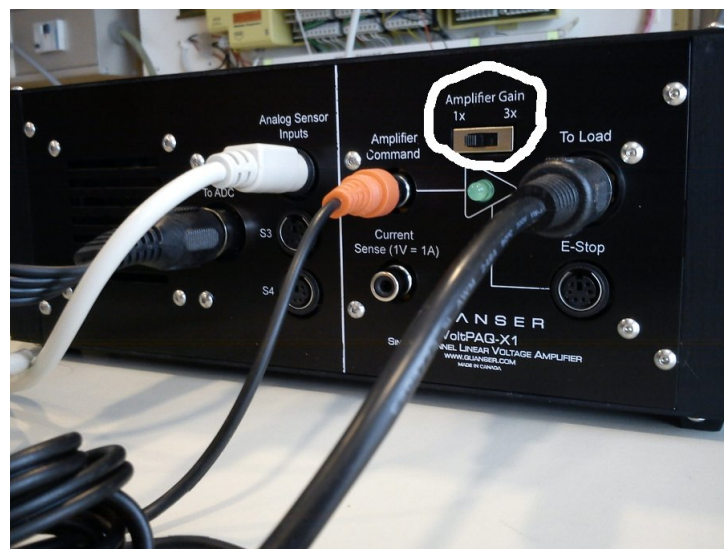
Figure 5: Amplifier Gain should be set to 1x.
