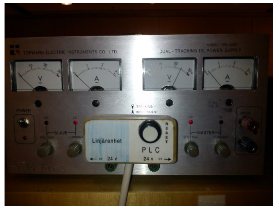
Figure 6: PLC power connected to DC power supply
