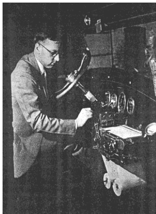
Figure 11. View of Highway Washboard Test Car of the Engineering Experiment Station; Car Is Shown with High Pressure Tires.
