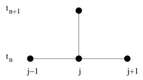
b) The system is solved numerically on a grid given by  $x_j = j\Delta x, j = 0, 1, 2...$  and  $t_n = n\Delta t, n = 0, 1, 2, ...$  using an explicit three-point scheme, see the figure below.
