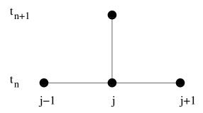
b) The system is solved numerically on a grid given by  $x_j = j\Delta x, j = 0, 1, 2...$  and  $t_n = n\Delta t, n = 0, 1, 2, ...$  using an explicit three-point scheme, see the figure below.
