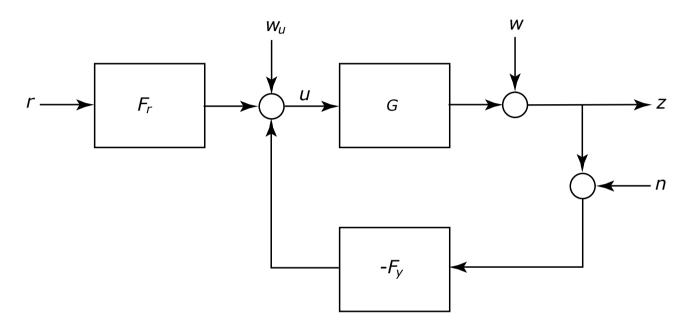
Controller: feedback  $F_y$ , feedforward  $F_r$
