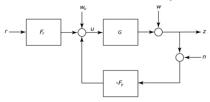
**Definition.** The closed loop system above is *internally stable* if it is input-output stable from  $r, w_u, w, n$  to all outputs u, z, y.
