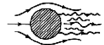
Turbulent boundary layer narrow turbulent wake (E)
