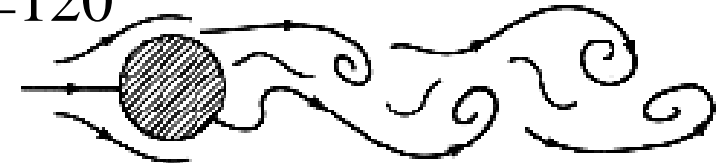
Oscillating Karman vortex street wake (C)
