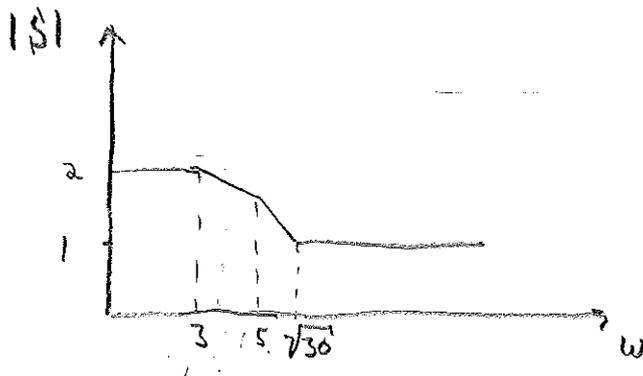
This basically means that we amplify low frequency disturbances and let high frequency disturbances pass through undamped.
