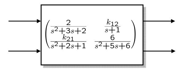
If  $k_{12}$  and  $k_{21}$  are small, it is convenient to use decentralized control – design controllers for loops in isolation
