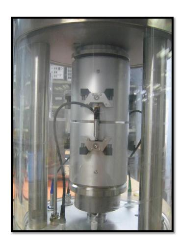
A dummy Sample (Proving ring) Should be run at the calibration certificate stress level to calibrate the instrument.
