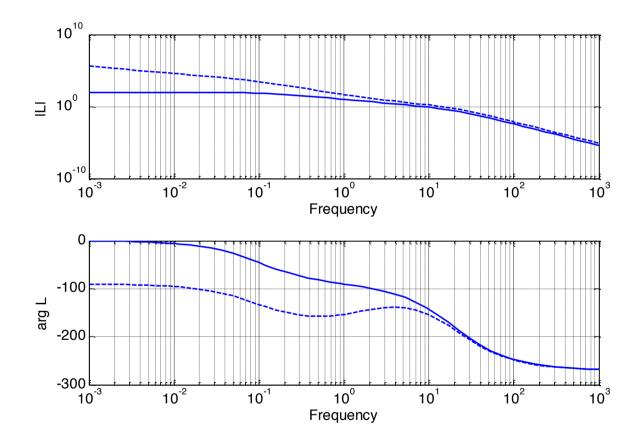
Low frequency gain, cross over ok, but poor phase margins.
