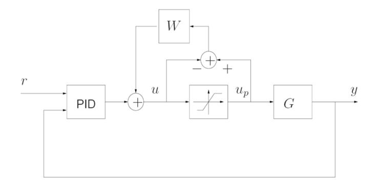
Common choice:  $W(s) = \frac{1}{sT_t}$  (tracking anti-reset windup) Rule-of thumb:  $T_t = \sqrt{T_i T_d}$  (T<sub>i</sub> integral time, T<sub>d</sub> derivative time of PID)
