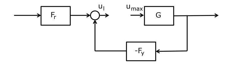
Constant input make plant and controller states to grow large ("wind up")
