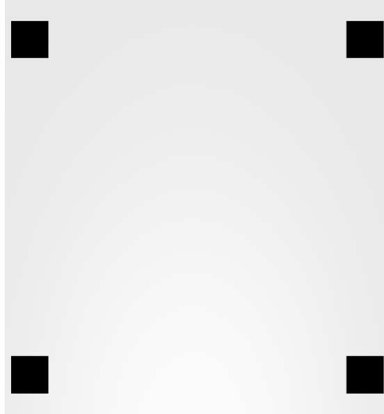
FIGURE 2.9: Unavailable area of an 80 \times 80 QR symbol
