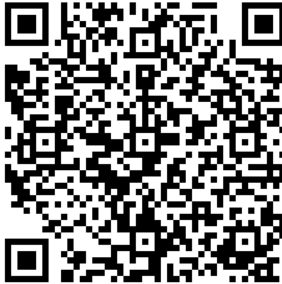
FIGURE 2.6: Data placement inside a QR symbol version 7 after applying masking
