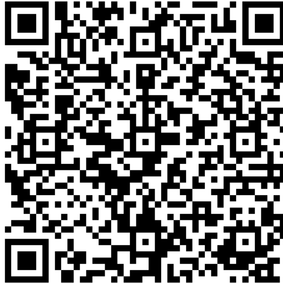
FIGURE 2.7: Final form of the encoded QR symbol version 7
